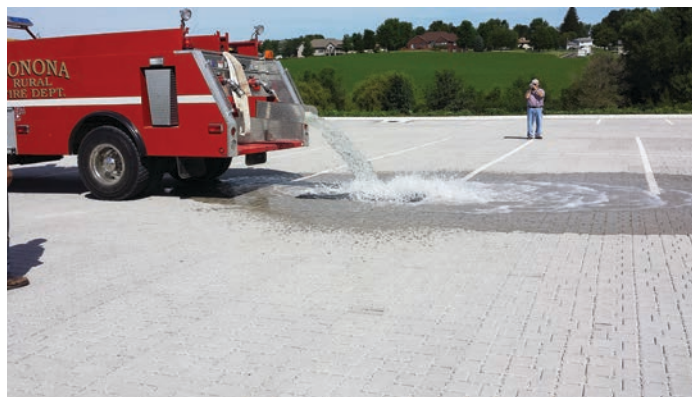
This fire truck gives a drainage demonstration at Monona, Iowa’s, aquatic center parking lot, which was improved with permeable pavers that allow water to seep down into the base. (Photo provided)
