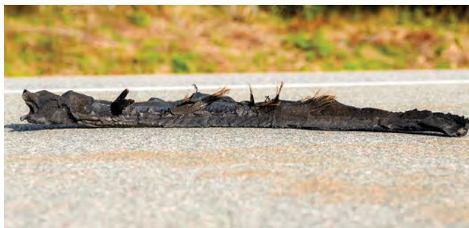
A common misconception about retread tires is that they are responsible for the "alligators," or the tire shreds, seen at the side of a roadway. These shreds are more often from newer tires that overheat because they don't have enough air. (Shutterstock.com)
