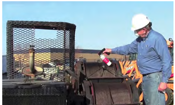
Aerosol greases will cover your equipment thoroughly and can help prevent the underapplying or overapplying of grease. (Photo provided by Lube-A-Boom)
