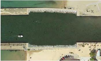
Pictured are wave absorbers being used by South Haven, Mich., to mitigate riverbank and lakefront erosion. (Photo provided)
