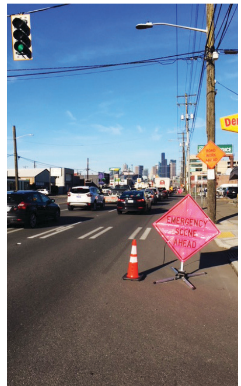
Fluorescent pink signs are used by the SRT to signal an incident ahead to drivers. Pink was chosen as a way to show motorists a difference between the incident scene ahead and a familiar orange construction zone sign. (Photo provided by Seattle Department of Transportation)
