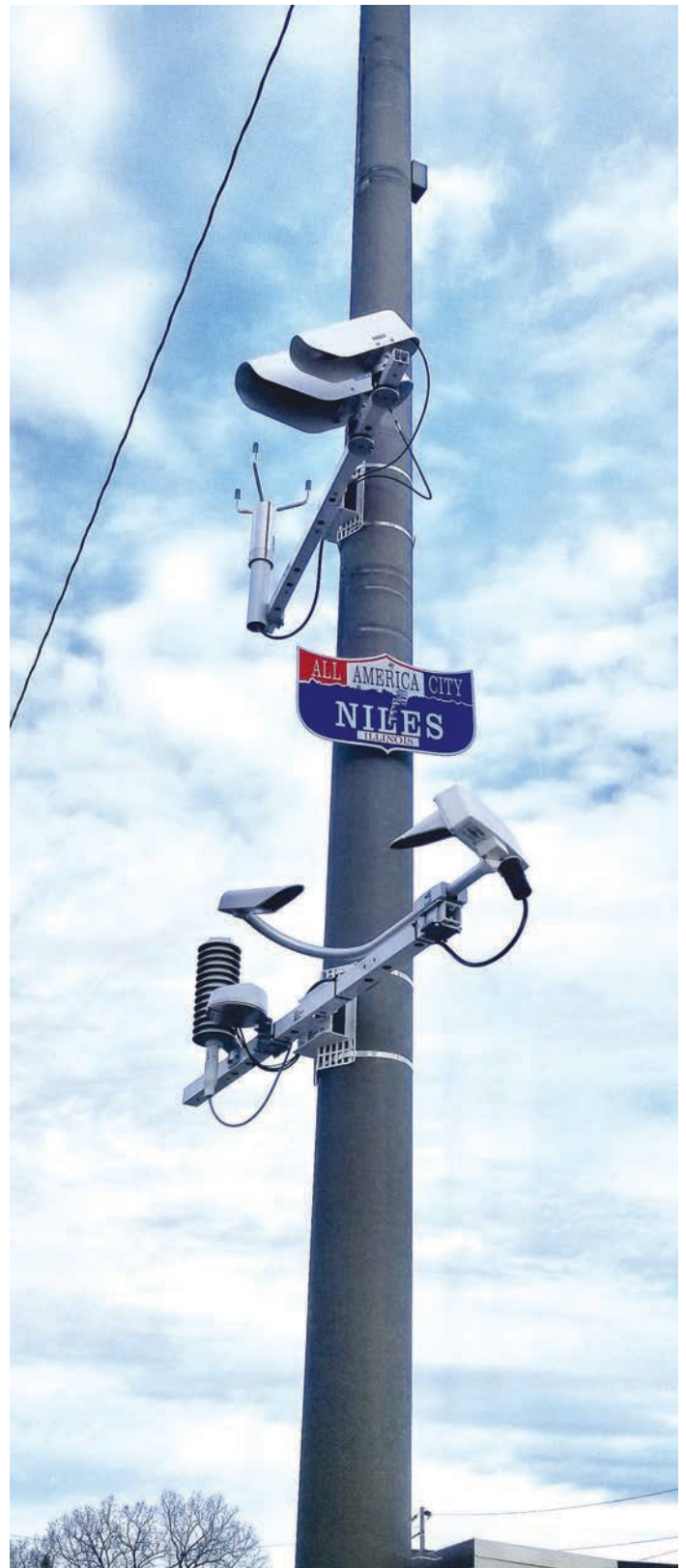
Pictured is one of the weather monitor sensors installed in the winter of 2018 by the village of Niles. It relays weather conditions, meaning the public works department isn’t reliant on a call from the police department when conditions are bad. (Photo provided)
