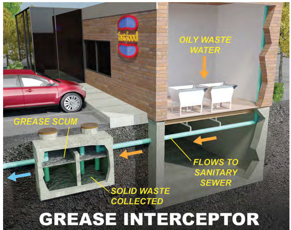
Grease traps and grease interceptors help to protect the sewer lines by catching the fats, oil, grease, solid waste and sediment before it can enter the public sewer lines. The traps and interceptors must then be emptied a minimum of every 90 days to keep them from facing a buildup. (Shutterstock.com)
