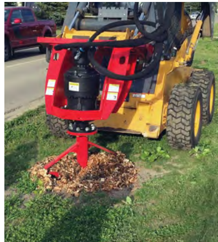
The Stumpex’s low RPM blades and vertical orientation create a safer environment when working around pedestrians or vehicles, as it dramatically reduces the likelihood of flinging material. (Photo provided)
