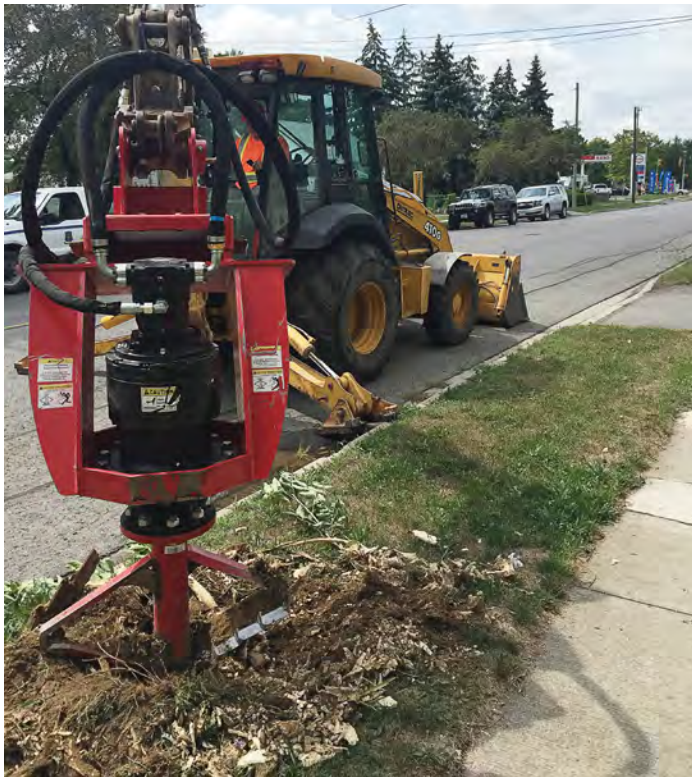
A 20- to 24-inch stump only takes 10-15 minutes to remove with Stumpex and leaves behind a small pile of large shavings that is easier to pick up. (Photo provided)
