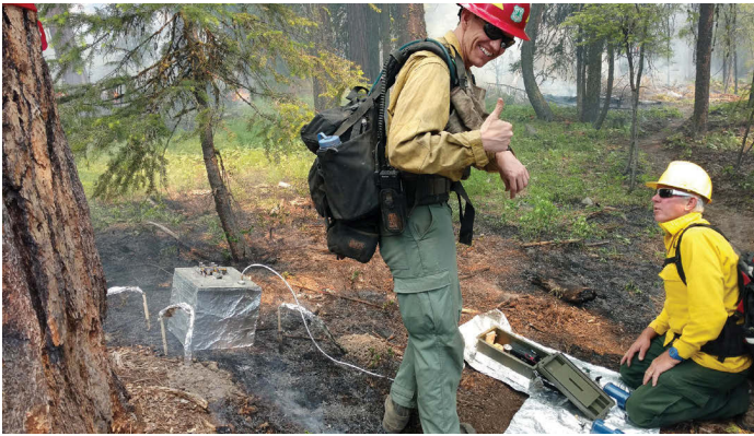
LEFT: Wesley Page, forestry technician, and Steve Baker, chemist, conduct research on smoldering fires. They are measuring the temperature at specific depths and consumption while collecting emissions samples of smoldering duff after a prescribed fire has burned through a small experimental plot in central Washington. The silver box is a portable chamber that fills with smoke for one minute and allows them to calculate the rate of carbon emission per unit area and to characterize the gases collected in the blue bottle. It is part of a Strategic Environmental Research and Development Program-funded study of smoldering combustion. (Photo by Matt Ellis)
