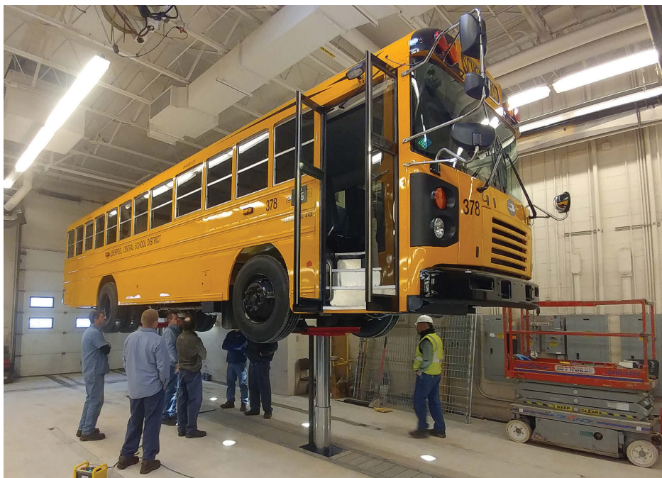
Complete access to the vehicle enables safe and efficient service and maintenance. Shown, maintenance workers inspect a school bus on Stertil-Koni's high-pressure telescopic piston lift, the DIAMONDLIFT. (Photo provided)
