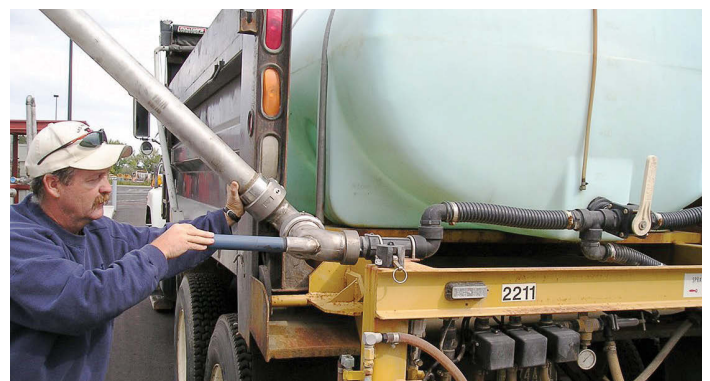
Crew Chief Keith Scott demonstrates a close-up of the quick attach setup. The truck loading island with quick attach setup features four loading arms for easy filling. Loading islands also feature hand-style hoses, all with 160 gallons per minute load time. (Photo provided by the city of Fort Collins, Colo.)
