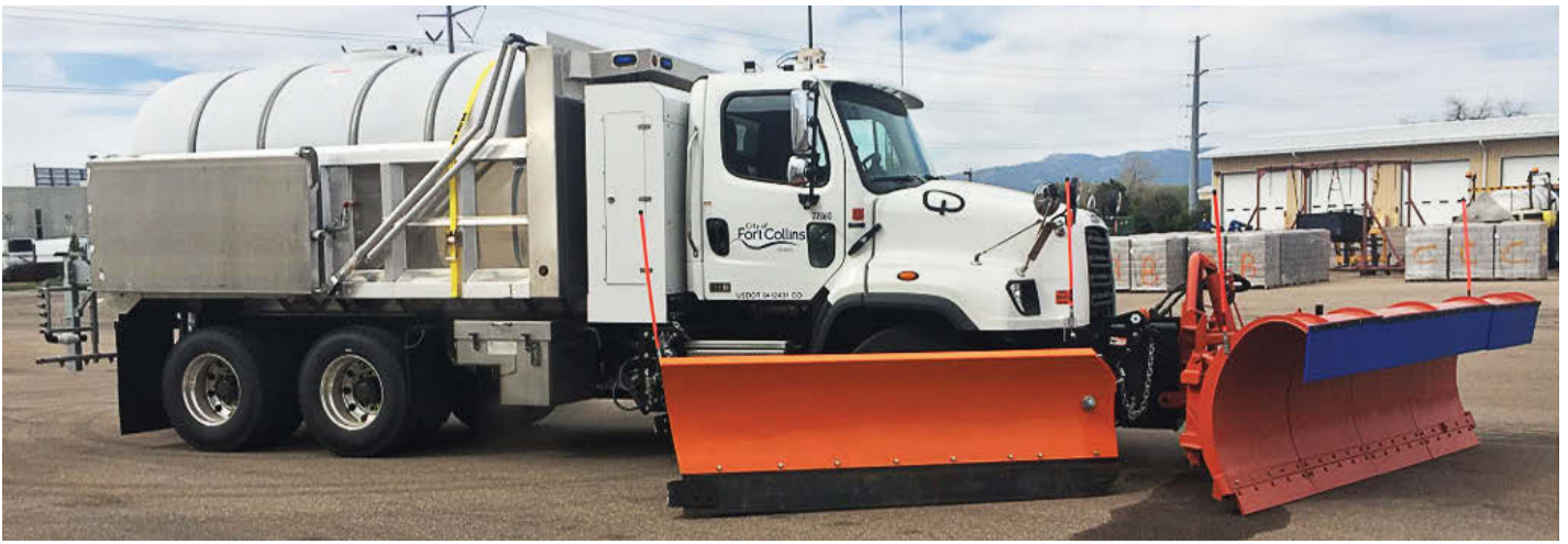
The city's compressed natural gas fleet is composed of eight tandem plow trucks that work throughout the snowstorms to keep the streets safe for residents. Each truck has a cost of about $370,000. Throughout the city of Fort Collins, Colo., there are 59 compressed natural gas vehicles. This is a typical CNG truck with a wing plow and liquid tank. (Photo provided by the city of Fort Collins, Colo.)
