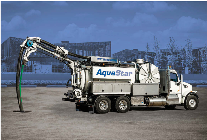
The AquaStar is equipped to clean sewer pipes as well as catch basins. (Photo provided)
