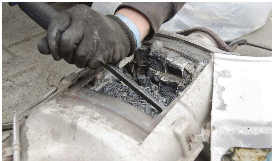
A mechanic removes a diesel particulate filter. Renewable diesel drops particulate matter emissions by 30 percent, meaning a longer duty cycle for particulate filters, less maintenance and less downtime. (Shutterstock.com)
