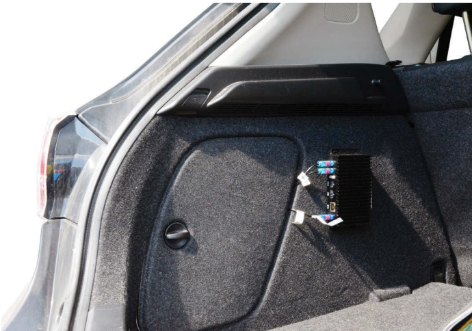
Pictured is the short-range radio unit that will be installed in the driver's truck or rear storage compartment. About the size of a paperback book, this equipment communicates with other CVs and devices. (Photo provided)
