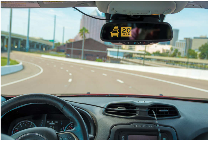
Drivers of connected vehicles on the Lee Roy Selmon Expressway's Reversible Express Lanes will receive an alert when traffic is backed up ahead. This warns the driver to slow down to a recommended speed as the vehicle approaches the end of a queue. (Photo provided)
