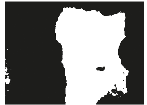
ABOVE and BELOW: These images show what a pothole will look like on the system when detected. In the raw data, the green and yellow shows a pothole on a road. In the system, the pothole is shown by the white area. (Photo provided)
