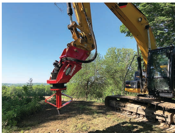
The Stumpex can be mounted on everything from traditional skid-steer type loaders, compact track loaders and rubber-tire backhoes to hydraulic track and wheel excavators with the new Stumpex EXC 20-ton model. (Photo provided)
