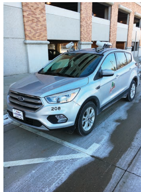
The SUV's $68,000-worth equipment includes four protruding cameras, two contour-measuring lasers, a GPS antenna, an onboard computer, image and symbol-recognition software and a printer. (Photo provided)
