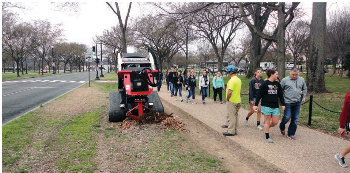
LEFT: The Stumpex can cut from 8 inches above ground to 8 inches below ground in less than four minutes. (Photo provided)
