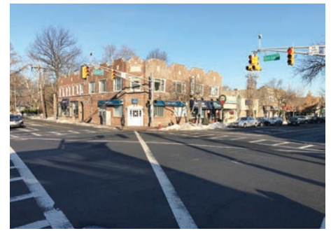
Very few people have complained about Leonia, N.J.'s, all-red phase traffic signal at the intersection of Broad Avenue and Fort Lee Road. Some have suggested that the wait time of 26 seconds should be reduced; however, most agree the wait is a small price to pay for pedestrian safety. (Photo provided)
