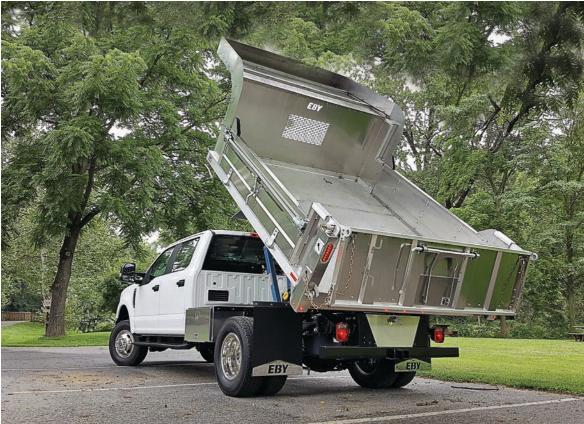
LEFT: EBY's all-aluminum flatbeds, dump bodies, stake bodies, service bodies and van bodies are lighter than steel, require less maintenance and are resistant to corrosion. Pictured is a general purpose dump body. (Photo provided)
