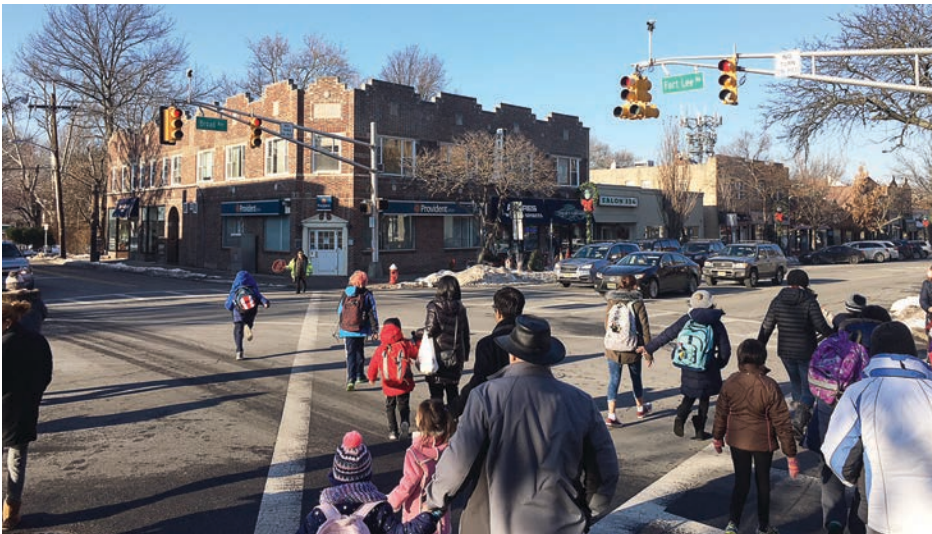
After a tragedy, Leonia, N.J., made a decision to turn a busy intersection into an all-red phase traffic signal. The signal stays red in all directions for 26 seconds every few minutes. (Photo provided)
