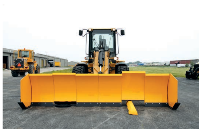
Independently moving moldboards "trip" over obstacles up to 9 inches in height and move below grade as well the same amount to contour to uneven surfaces.
