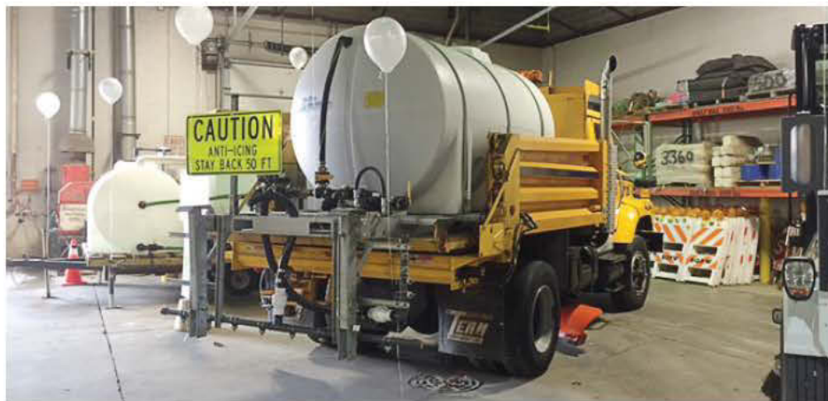
A liquid anti-icing truck is ready to go out. The village has invested in targeted trucks, specifically designed for snow removal; this has allowed for an increase in the amount of liquid application, which has reduced the amount of road salt applied. (Photo provided)
