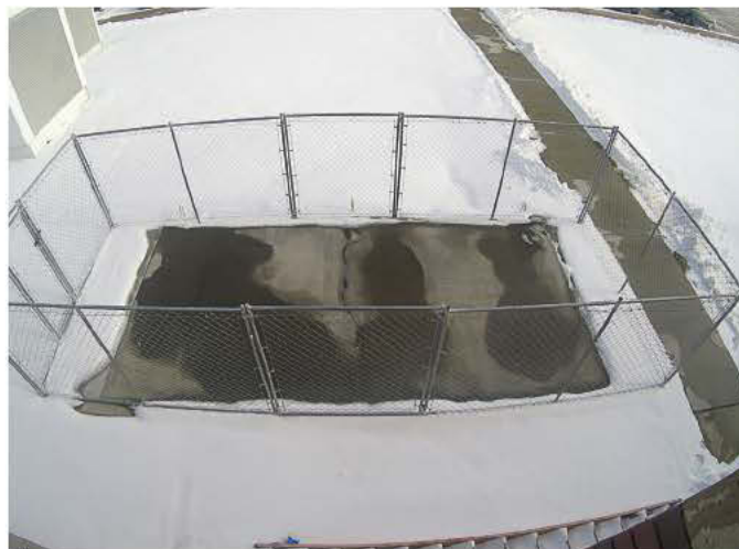
This photo is actually from a four-hour time-lapse video showing conductive concrete melting fresh snow from its surface during a winter storm in Omaha in December 2015. (Photo provided)
