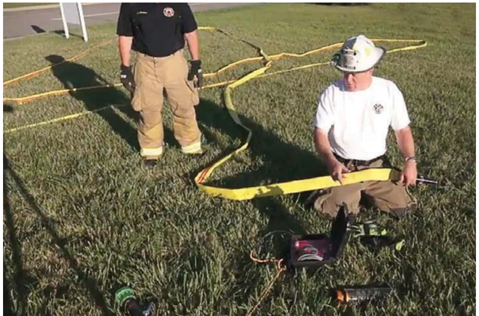
Allen monitors gallons per minute using a flow meter. (Photo provided)
