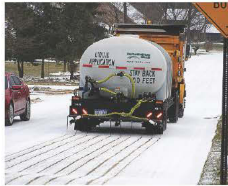
Plows directly apply the brine to snowy roads in Farmington Hills, Mich. (Photo provided)
