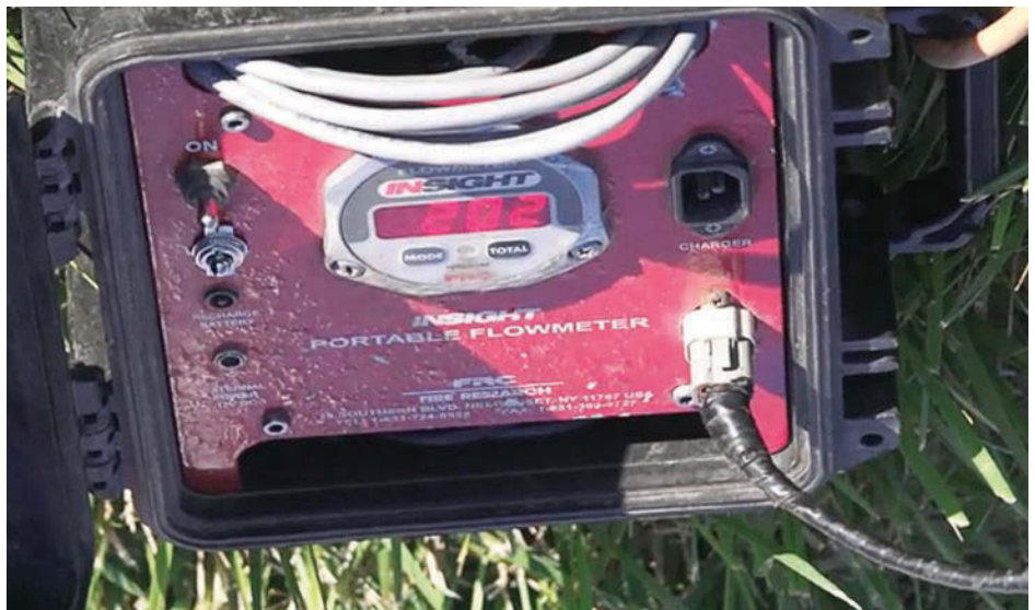
A portable flowmeter relays the actual flow, which might not actually be the amount fire departments think they are pumping. (Photo provided)
