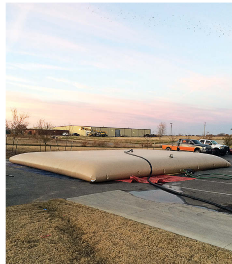
Beyond firefighting products, Husky Portable Containment also offers other solutions. Pictured is the field test of a 50,000-gallon bladder tank being used as a drinking water supply while a small town had its water tower repaired. (Photo provided)
