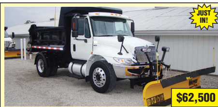
2008 INTERNATIONAL 4300 DT466, Allison auto, air brakes, Under CDL, new snow plow pkg., including central hydra, 10' plow and stainless tail gate sander
