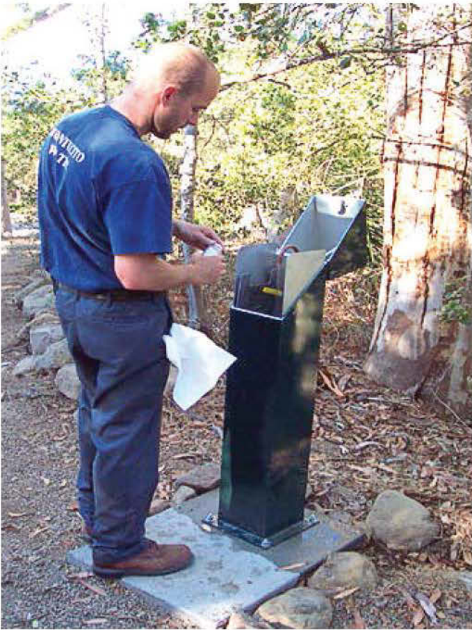
A technician draws a water sample from a water sampling station; water sampling stations reduce chances of receiving a false positive when testing water. (Photo provided)
