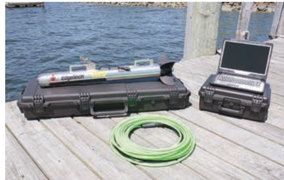
LEFT: Deployment of a side-scan sonar system by a Department of Natural Resources entity. (Photo provided)
