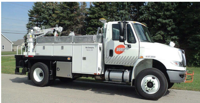
ABOVE: Here, the all-new 2,000-pound Venturo ET6K service crane is mounted on a We Energy service truck in Wisconsin. The ET6K allows operator use without needing the new 2017 crane certification. (Photo provided)
