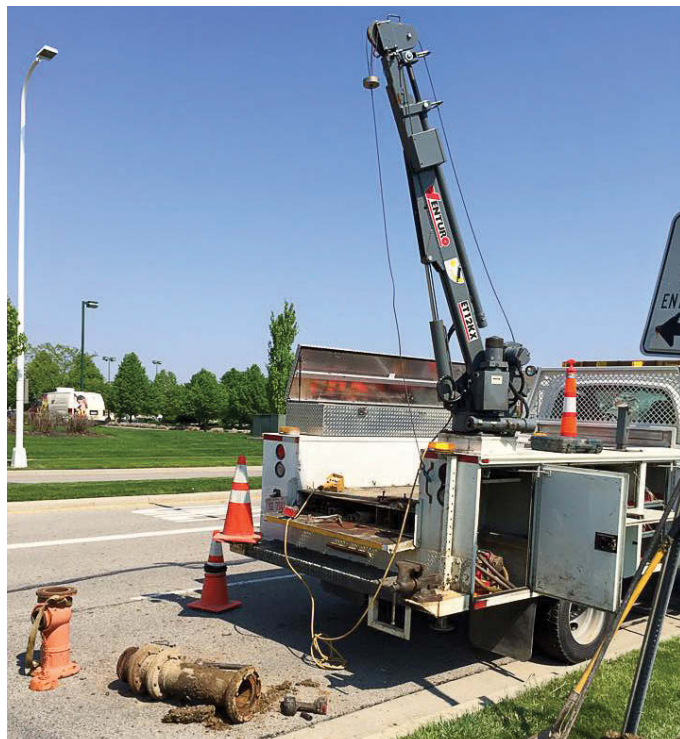
ABOVE: Here, the all-new 2,000-pound Venturo ET6K service crane is mounted on a We Energy service truck in Wisconsin. The ET6K allows operator use without needing the new 2017 crane certification. (Photo provided)
