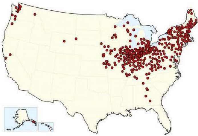
There are currently more than 700 CSOs in use in the United States. When it rains, such systems are often unable to contain the capacity, resulting in overflows into local waterways. (Image provided)
