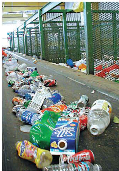
At Boulder County Recycling Center's paper sorting line, employees catch items that may hurt the machinery if they were to get through. Recycling centers like this one use a combination of automated systems and manual labor to separate recycled materials before they are sold to manufacturers. (Photo provided)
