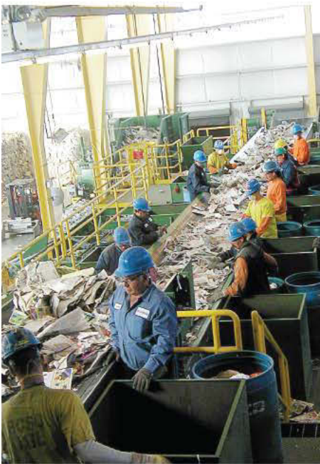
At Boulder County Recycling Center's paper sorting line, employees catch items that may hurt the machinery if they were to get through. Recycling centers like this one use a combination of automated systems and manual labor to separate recycled materials before they are sold to manufacturers. (Photo provided)
