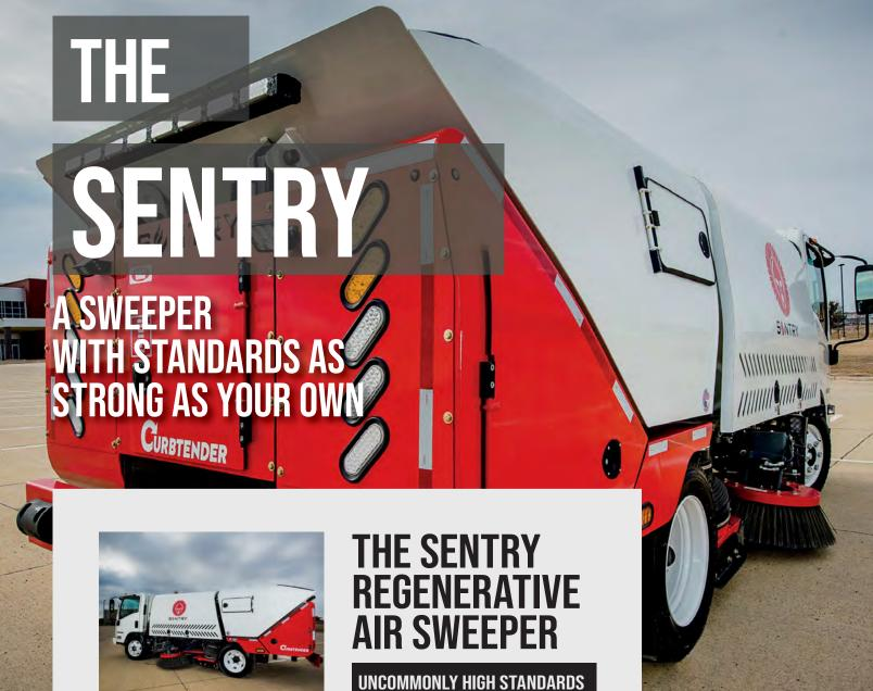
Under CDL platform with over CDL performance. In-cab control of gutter broom speed, pressure, and angle. Hopper and fan are made entirely of Hardox® 450 abrasion resistant steel designed to stand up to the abuse of debris. Crescent shaped pick up head funnels debris to the center of machine. On-screen diagnostics keep information at your finger tips and makes it easier to maintain your sweeper.
