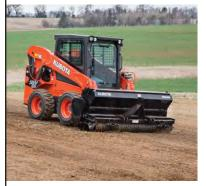
and Primary Seeders all feature proven fluted seed cups to precisely meter seed in a broadcast pattern and a notched iron packer roller insures good seed to soil contact. Visit landpride.com to locate a dealer and ask for a Sourcewell quote.
