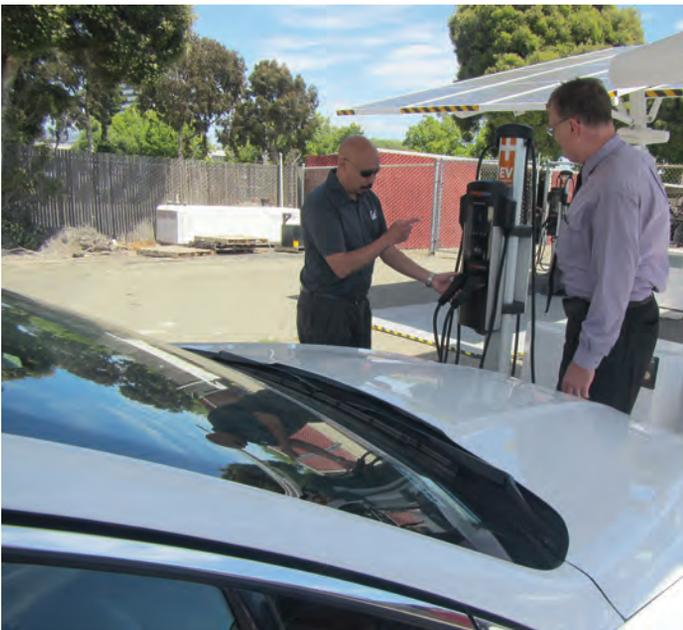
From left, Jason Chin, Oakland's fleet compliance coordinator, and Richard Battersby, interim assistant director of Oakland's bureau of infrastructure and operations, check out one of the EV ARC self-contained, solar-powered Level 2 charging stations. Electric cars charged at it will be using 100 percent renewable fuel. (Photo provided)
